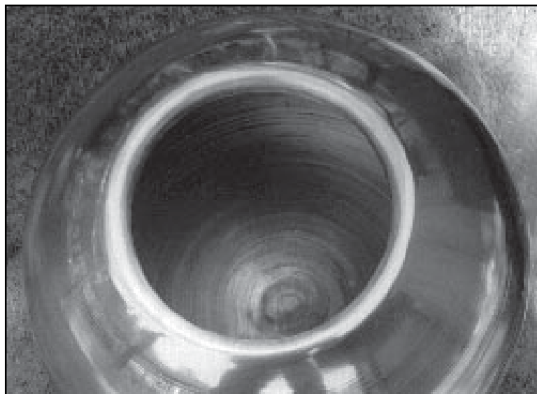
Fig. 19 - Bottom of Collector , showing radiused column entrance hole.
