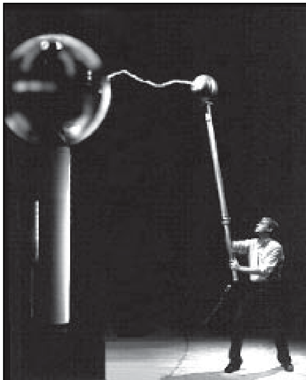
Fig. 2 - This science-show Van de Graaff Generator can deliver a spark over 48" long. The generator is 10' tall and has a 42" diameter collector. The author constructed the machine in 1988 for The Science Place museum in Dallas, Texas.
